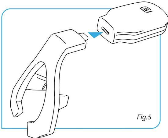
To start using eXcite<sup>OSA</sup>, connect the mouthpiece to the control unit as shown on Fig 5.
